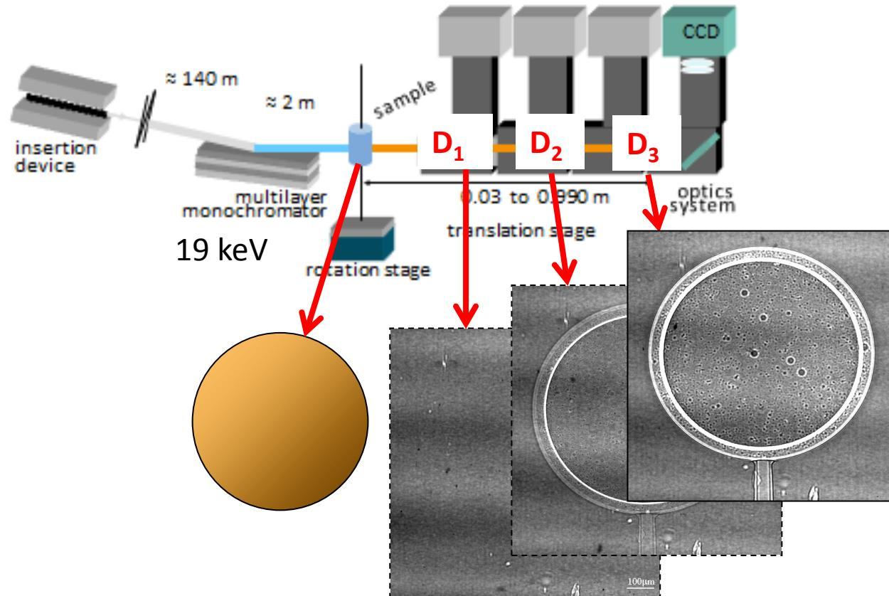
Phase contrast increases with the propagation distance
