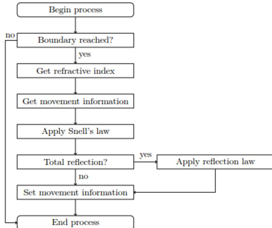
FIGURE 3.1: A schematic of the XrayBoundary process.
