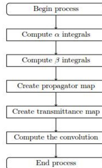
FIGURE 3.2: A schematic of the Fresnel diffraction actor algorithm.
