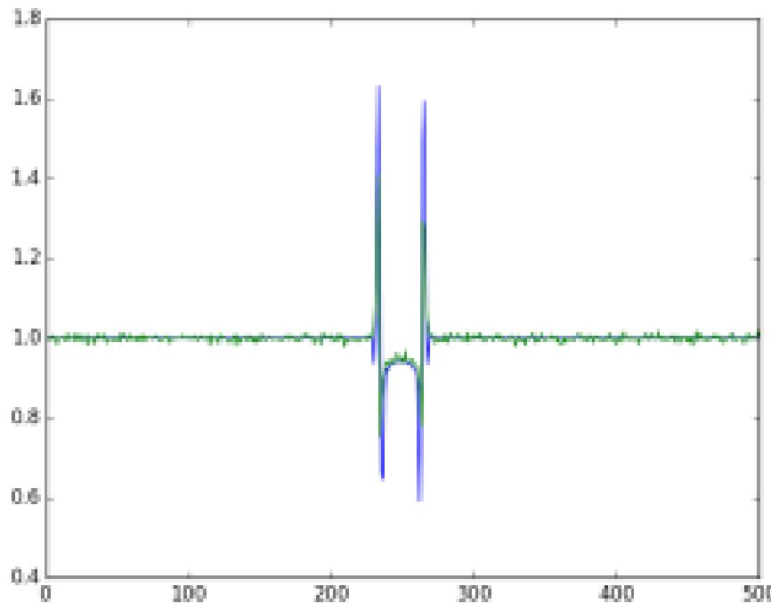
FIGURE 3.8: Comparison of the profiles of the stochastic model and the analytical model. The green curve is obtained using the Monte Carlo refraction model. The blue curve is obtained using the analytical Fresnel diffraction model
