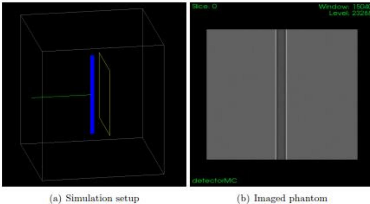
FIGURE 3.7: The phantom is an aluminium wire (blue) which has a radius of  $15.208\text{ }\mu\text{m}$ . The refractive index decrement of aluminium at  $19\text{ keV}$  is  $\delta = 2.0 \times 10^{-6}$ . To capture the image, we use a flat panel detector (yellow) with a pixel size of  $1\text{ }\mu\text{m}$ . For the sake of simplicity, only one photon's movement is showed (green).
